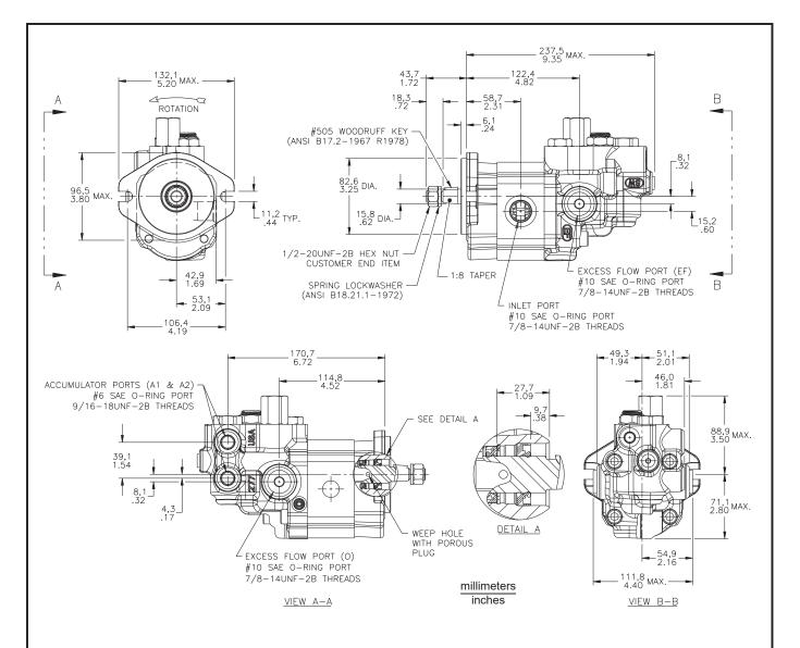
NOTE: Dimensions shown are for a model number which features SAE "A" 2-bolt flange mounting with SAE "A" 1:8 tapered shaft. Other options are available. Contact ZF Off-Highway Solutions Minnesota Inc. for more information.
