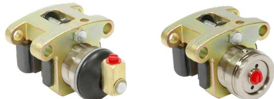
The 515 **Spring Apply, Hydraulic Release** design uses a stack of Belleville springs to apply the brake and hydraulic pressure from a source such as a master cylinder to release the brakes. This design can be used with a rotor 5/16 to 1/2 inch thick having a diameter of 6 inch or larger.
