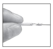
2. Grasp the crimped contact approximately 25.4 mm (1.0 in) behind the contact barrel.
