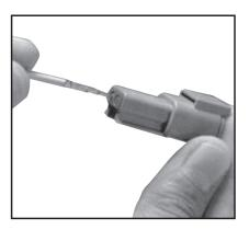
3. Hold the connector with the rear grommet facing you.
